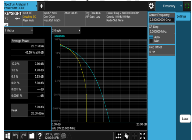
Band41 20MHz 64QAM RB100 0 CH41490
