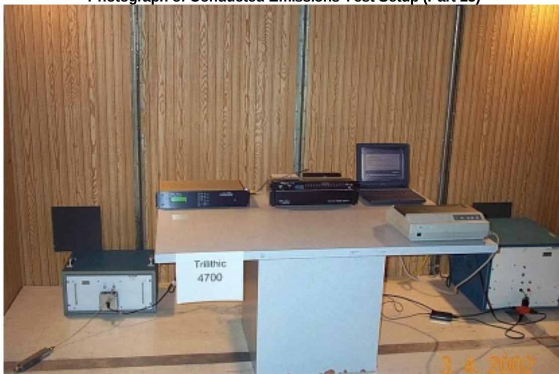
Photograph of Conducted Emissions Test Setup (Part 15)
