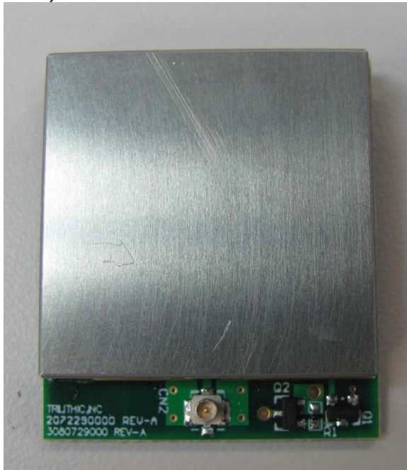
2) Wi-Fi Module with top Shield removed; still has inner shield.
