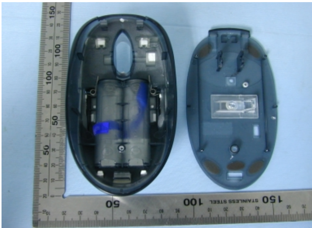
Case Inside View of EUT
