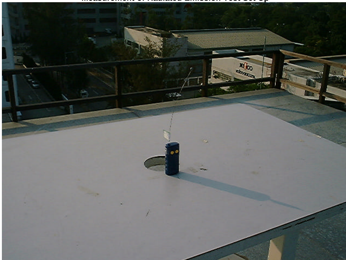
Measurement of Radiated Emission Test Set Up
