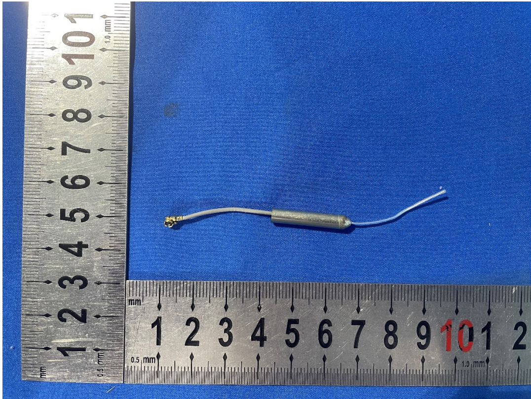
Photo 3: Internal View for 2.4G-WiFi/BLE Antenna
