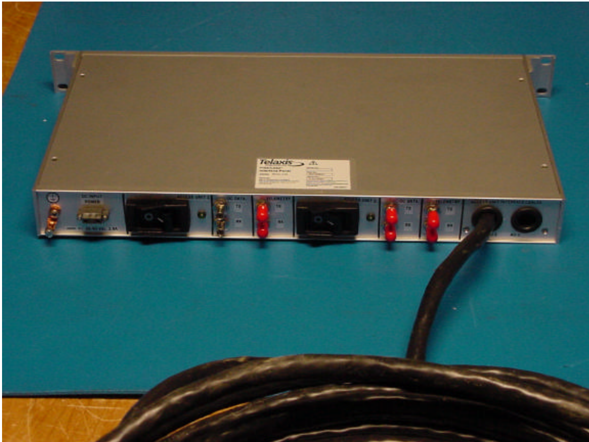
PHOTOGRAPH 13: FIBER BREAKOUT BOX REAR VIEW
