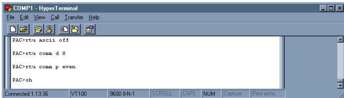
Figure 20: Configure TPAC for Modbus RTU
