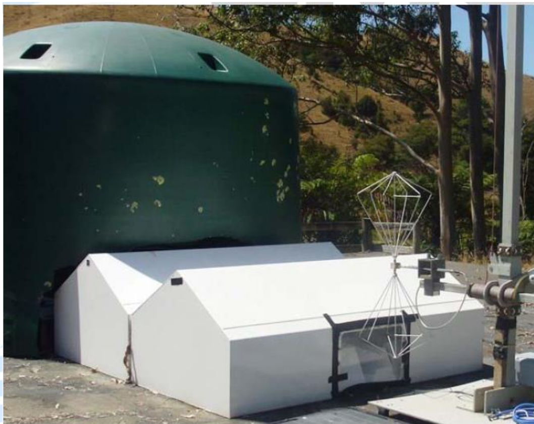
Test Shed showing the use of a Log Periodic Antenna
