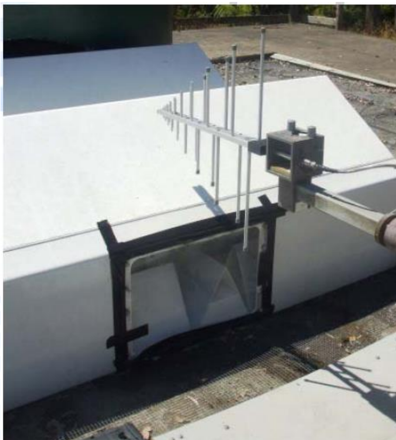
Test Shed showing the use of a Horn Antenna
