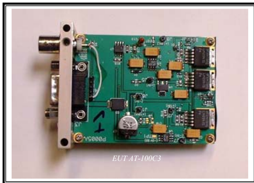
Fig 10. AT-100C3 Power Supply
