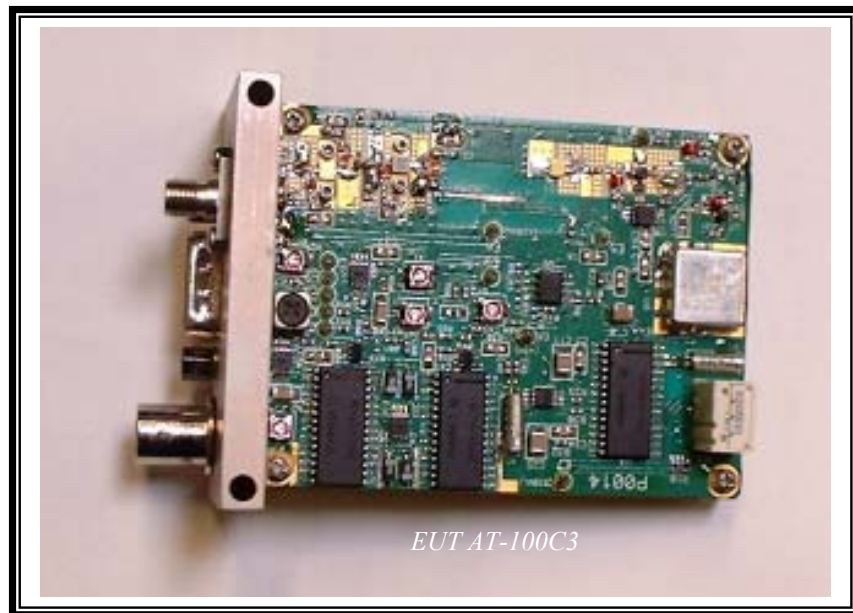
Fig 9. AT-100C3 RF Board
