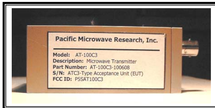
Fig 5. Metallic Equipment ID label affixed to AT-100C3
