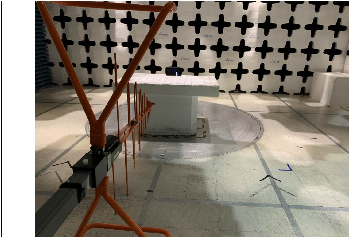
Radiated Emission Test 30MHz-1GHz Front View
