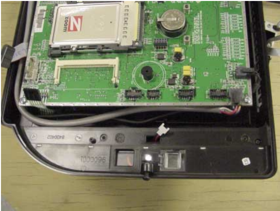
Inside of EUT, white connector on bottom of photo goes to antenna.
