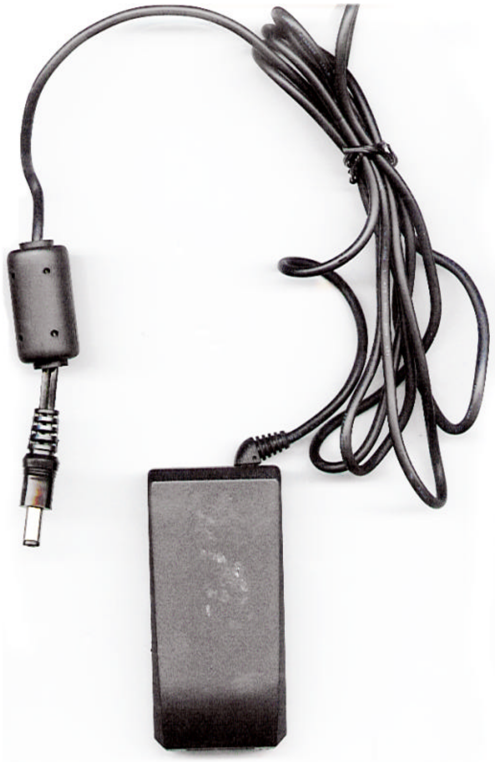
POWER SUPPLY UPPER VIEW
