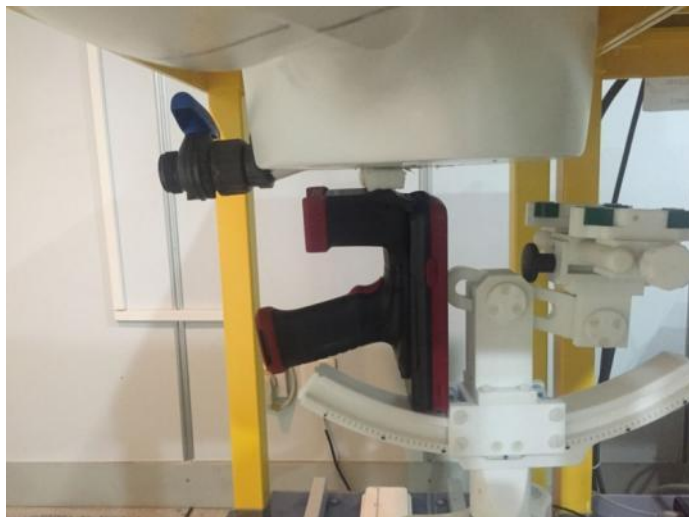
Fig.13 Body Edge A(UP,10mm separation)
