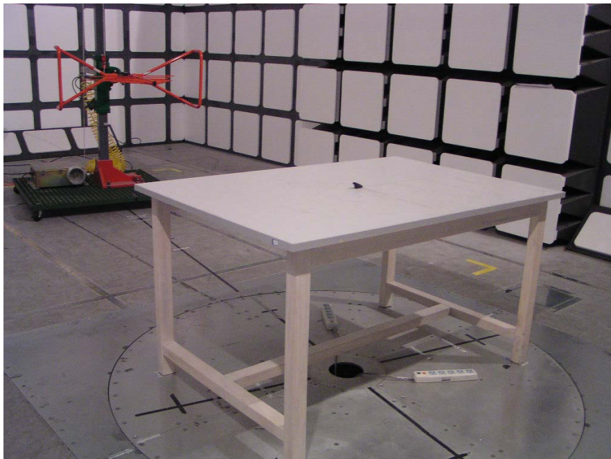
Radiated Emission - Rear View (30 MHz-1 GHz)
