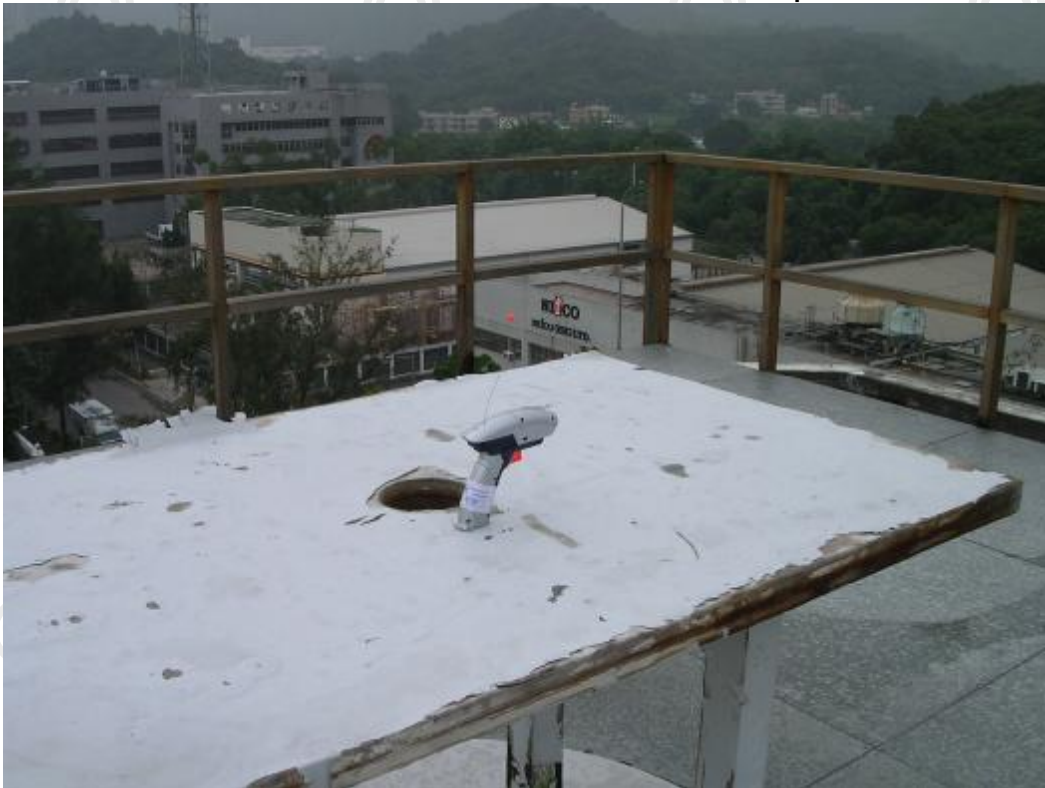
Measurement of Radiated Emission Test Set Up
