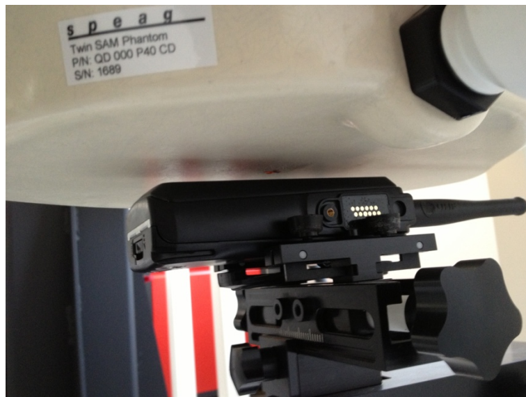
10mm Face-held, The EUT display towards phantom
