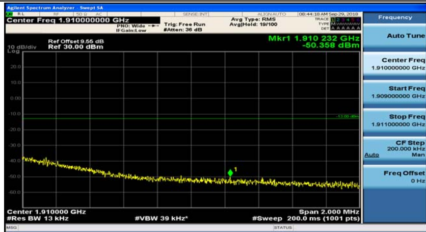
(Channel Bandwidth: 5 MHz)_HCH_QPSK_1RB#24
