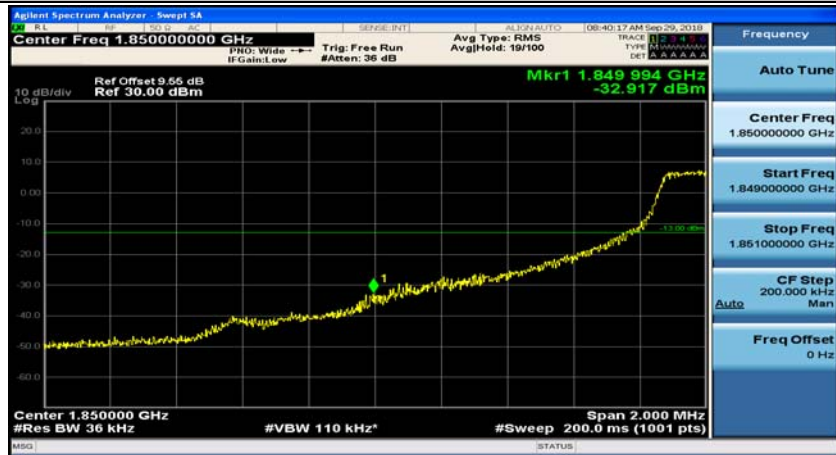
(Channel Bandwidth: 3 MHz)_LCH_16QAM_8RB#7
