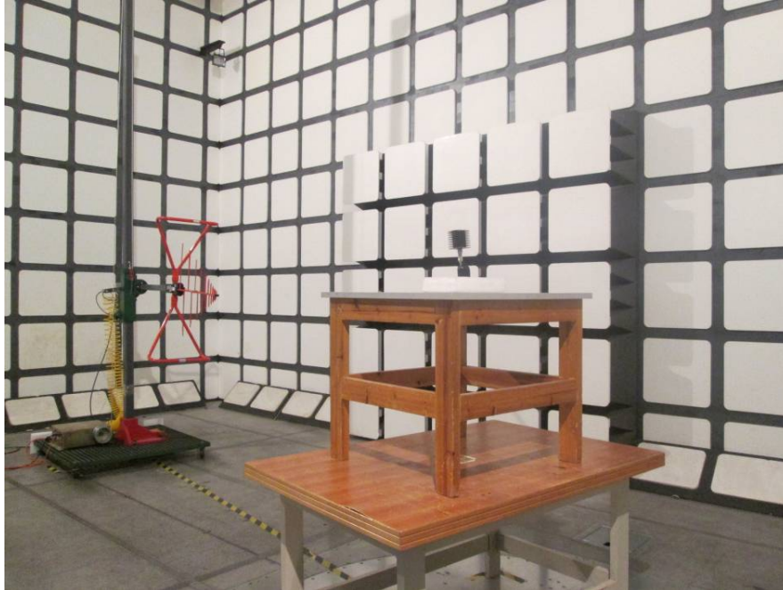
Transmitting Radiated Emissions (Below 1 GHz)
