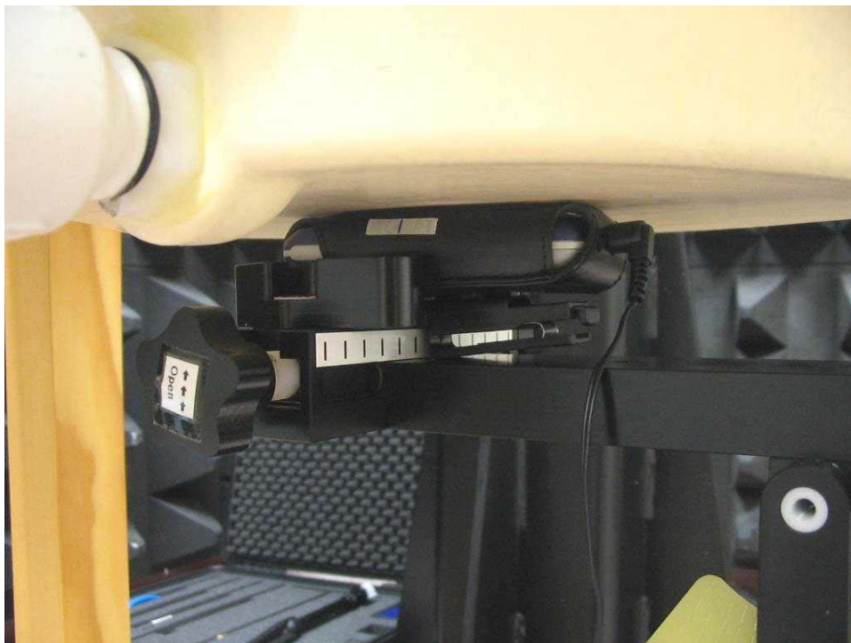
SAR Test Setup At Flat Phantom – Closer View (EUT Front Touched Phantom)
