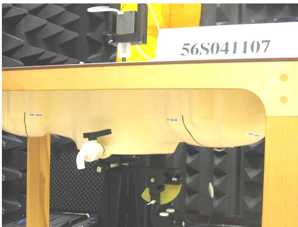
SAR Test Setup At Flat Phantom
