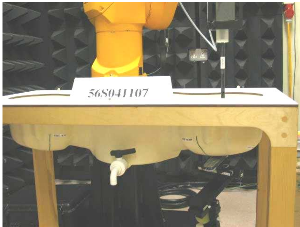
SAR Test Setup (Device at Head Phantom)
