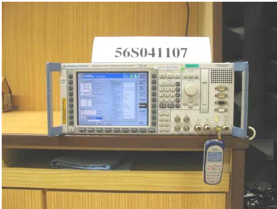
Conducted Power Measurement Setup – Far View
