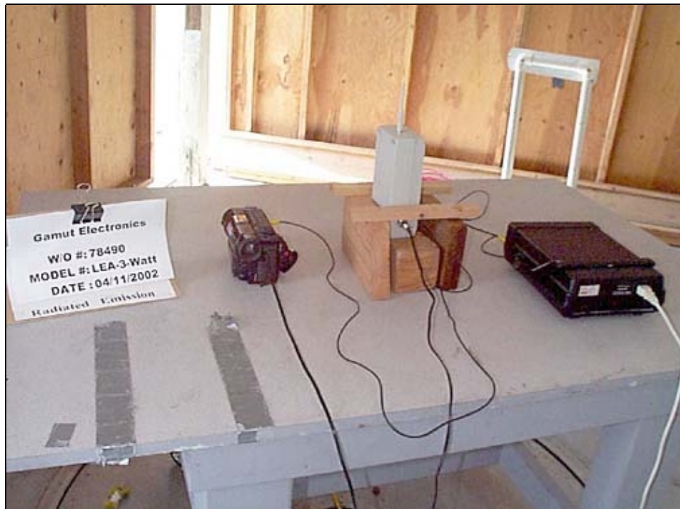
OATS Test Setup - Back View
