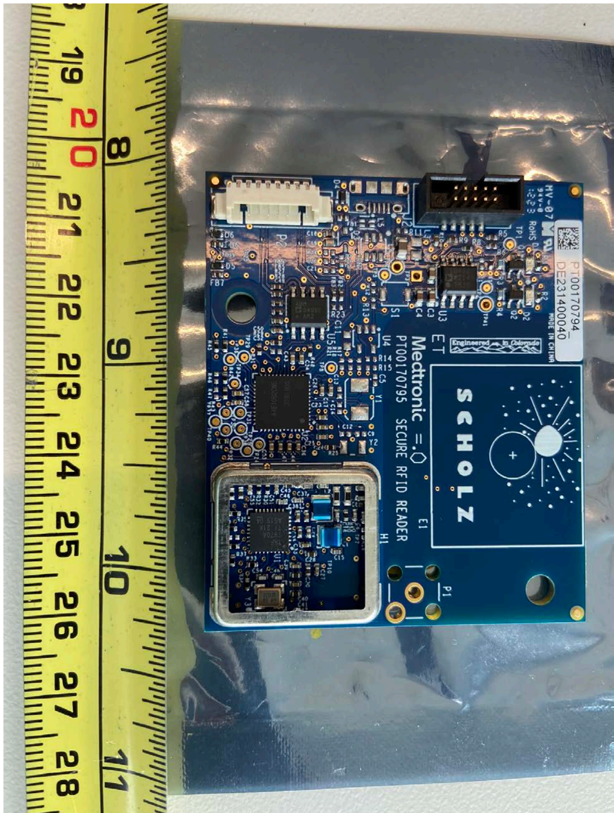
Figure 2: Module Top view Shielding removed
