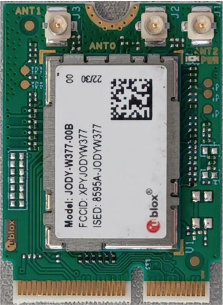
Figure 1: Radio module close-up photo - Top View
