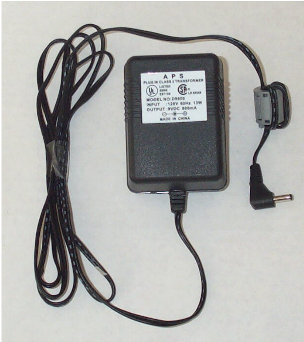
Transformer Provided with EUT
