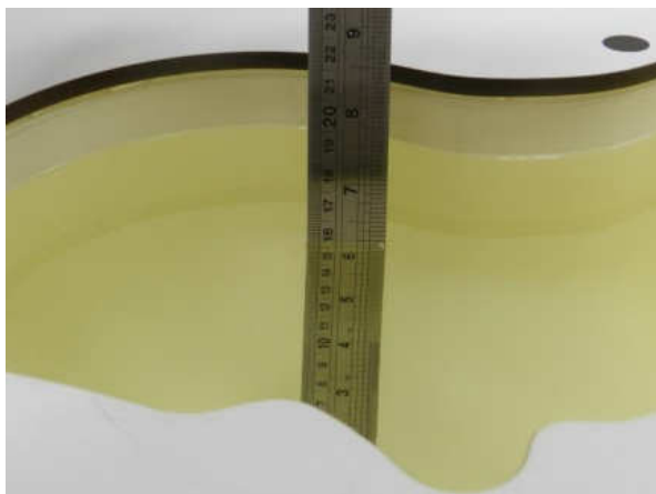
Fig 10.1 Photo of Liquid Height for Head SAR
