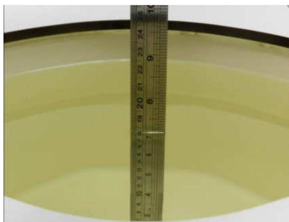
Fig 10.2 Photo of Liquid Height for Body SAR
