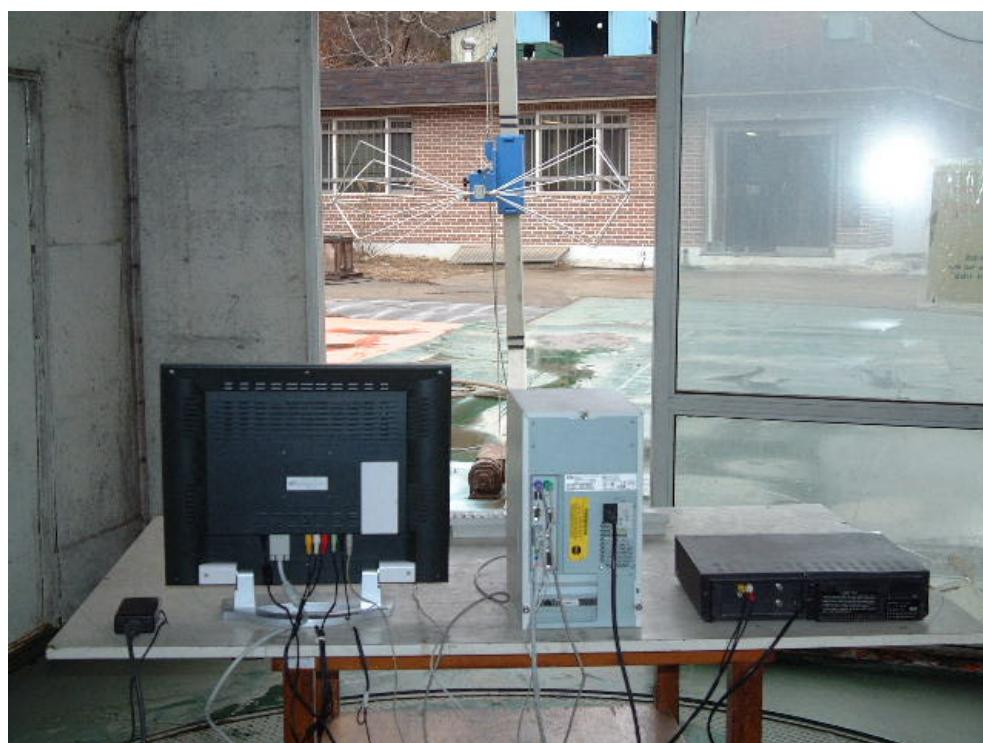
RADIATED EMISSION SETUP PHOTOGRAPH - REAR VIEW ( 30 - 300 MHz )
