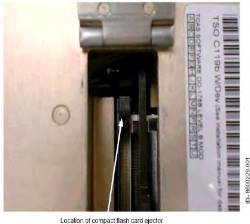
Figure 5-6: Compact Flash Card Ejector Location
