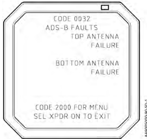
Figure 6-20: ADS-B Fault Page 3 (Code 0032)
