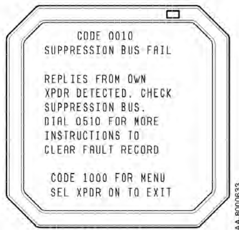
Figure 6-11: Suppression Bus Fail Page
