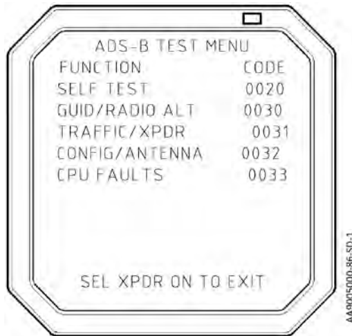
Figure 6-16: ADS-B Test Menu Page (Code 2000)
