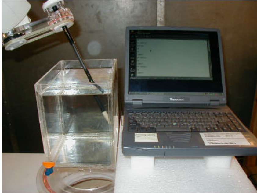
Figure S8. Configuration 1 per Table 10 (Antenna separated from box phantom by 15 mm)
