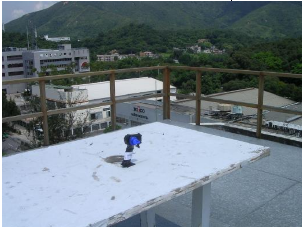
Measurement of Radiated Emission Test Set Up
