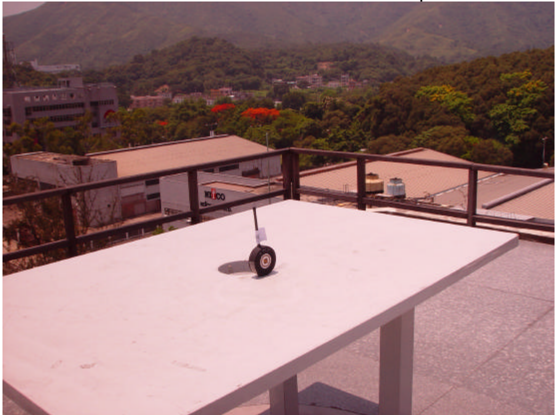
Measurement of Radiated Emission Test Set Up
