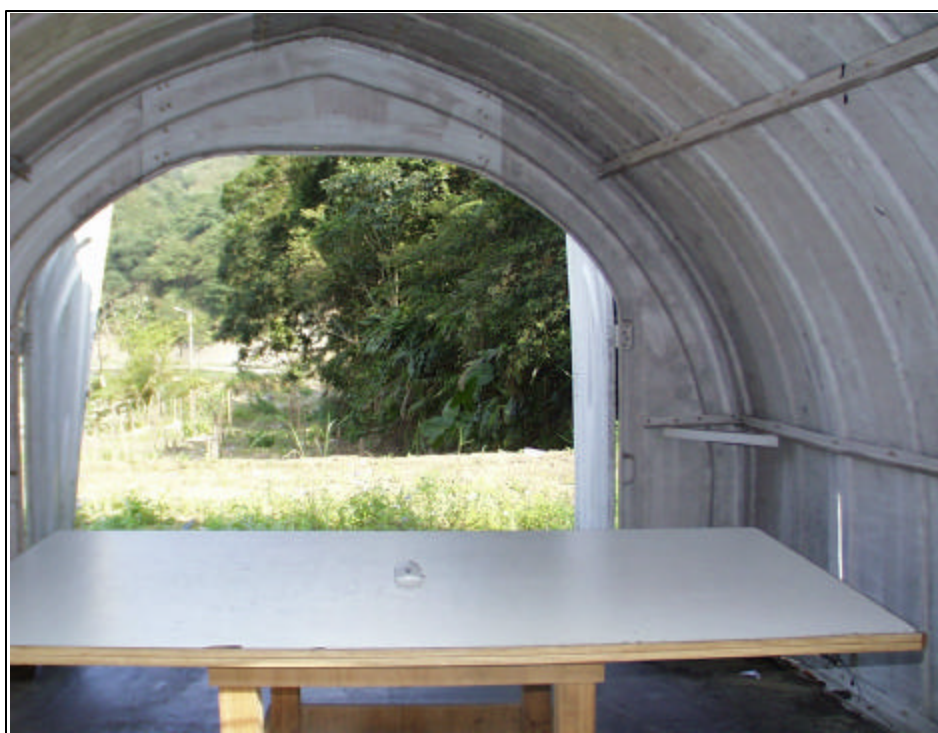
Radiated Open Site Test Set-up
