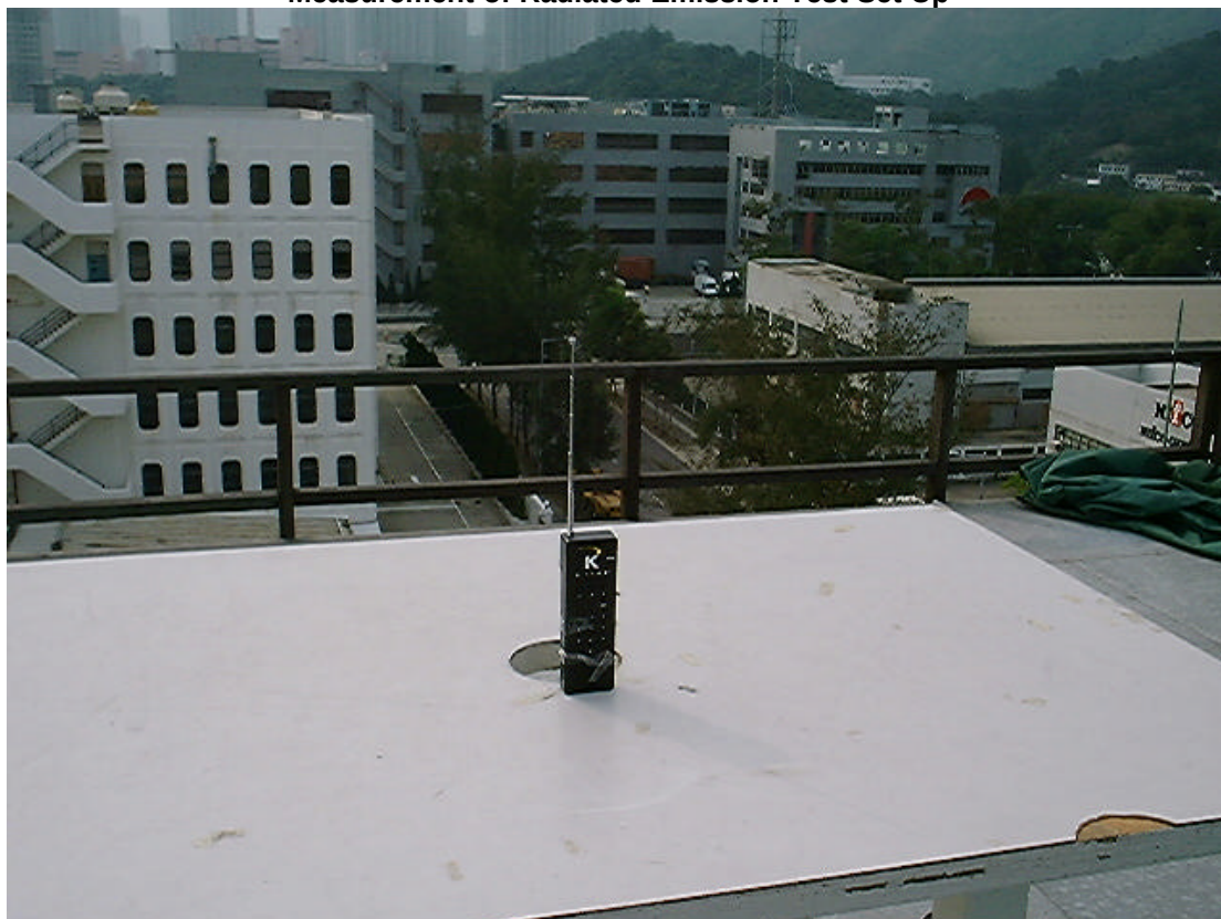
Measurement of Radiated Emission Test Set Up
