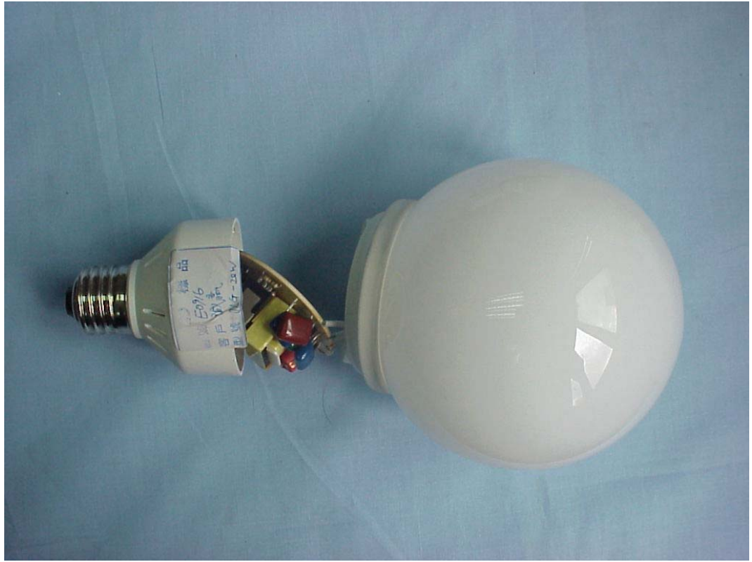
FIGURE 4 ENERGY SAVING LAMP (M/N: JLG-20W) COVER REMOVED
