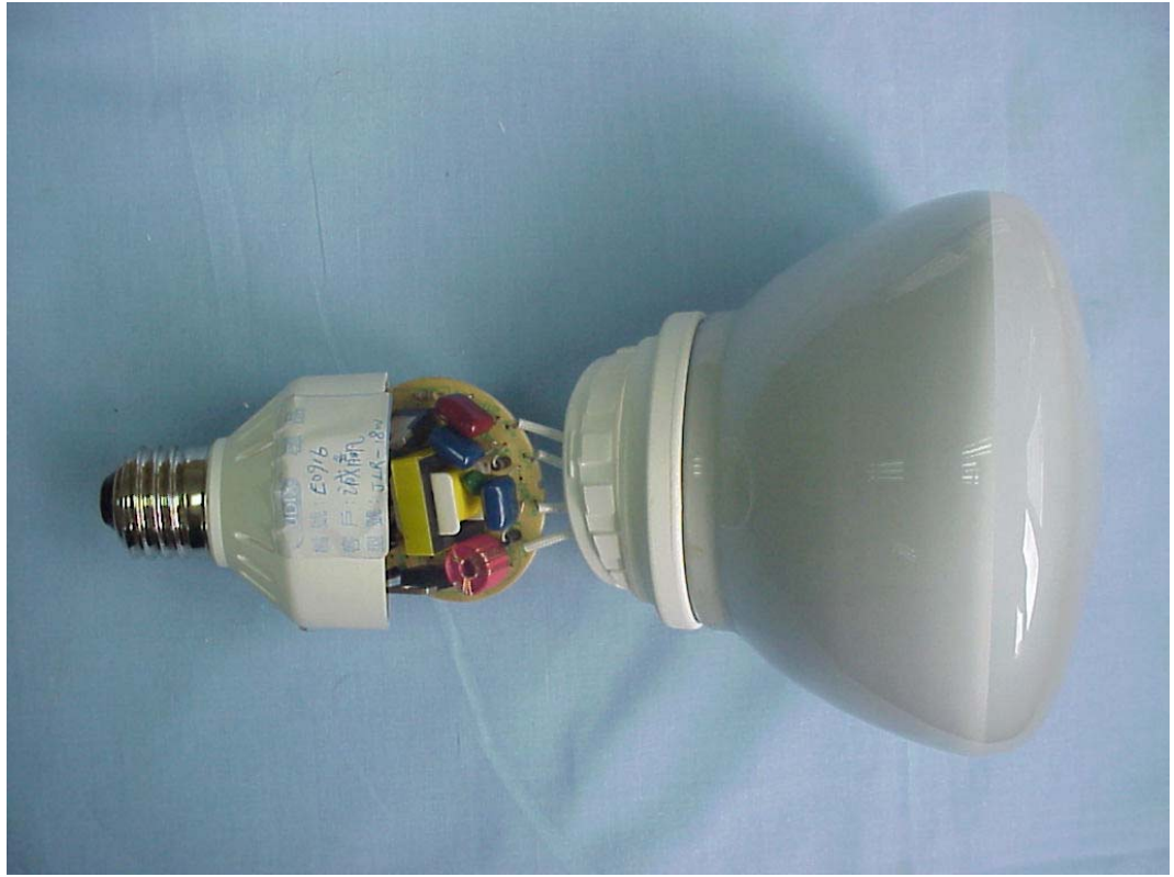
FIGURE 25 ENERGY SAVING LAMP (M/N: JLR-18W) COVER REMOVED
