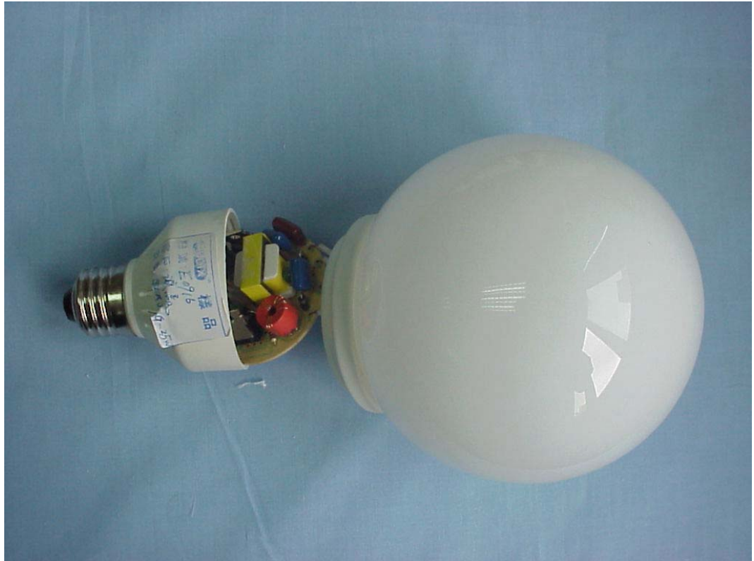
FIGURE 10 ENERGY SAVING LAMP (M/N: JLG-25W) COVER REMOVED
