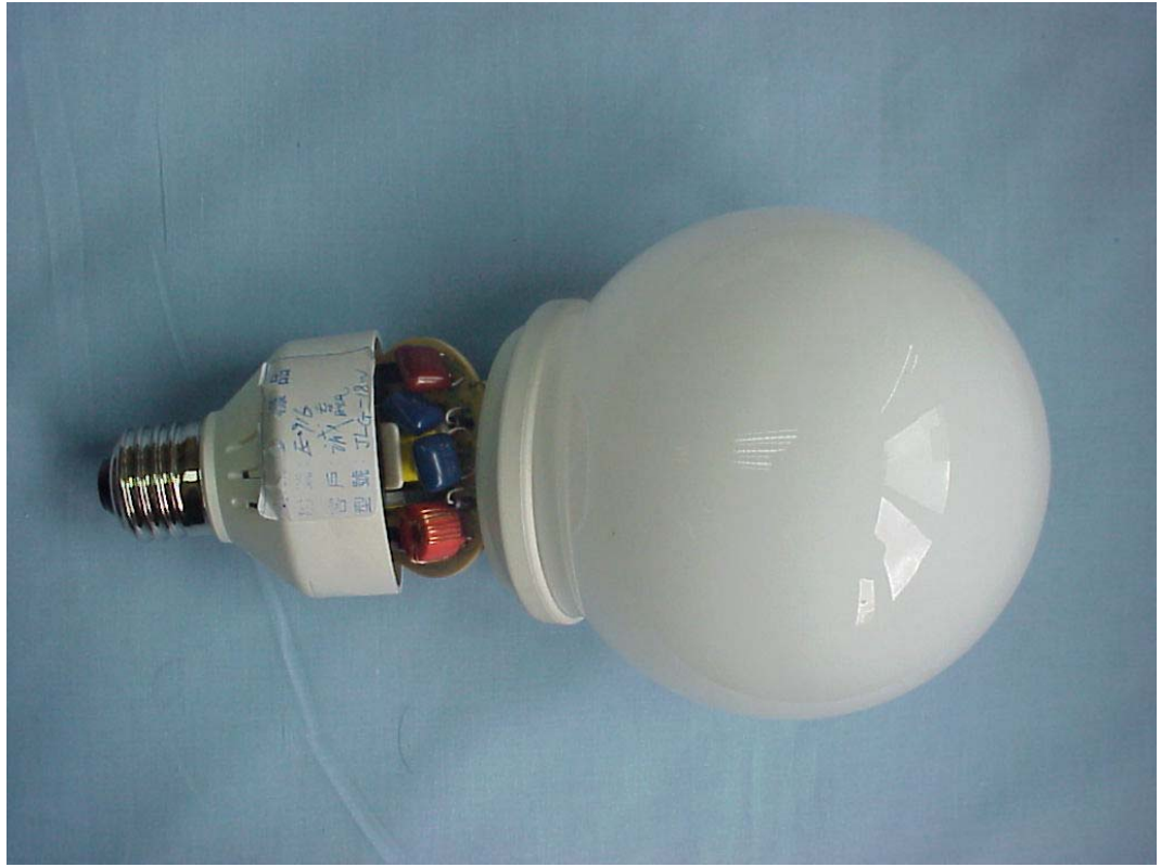
FIGURE 1 ENERGY SAVING LAMP (M/N: JLG-18W) COVER REMOVED
