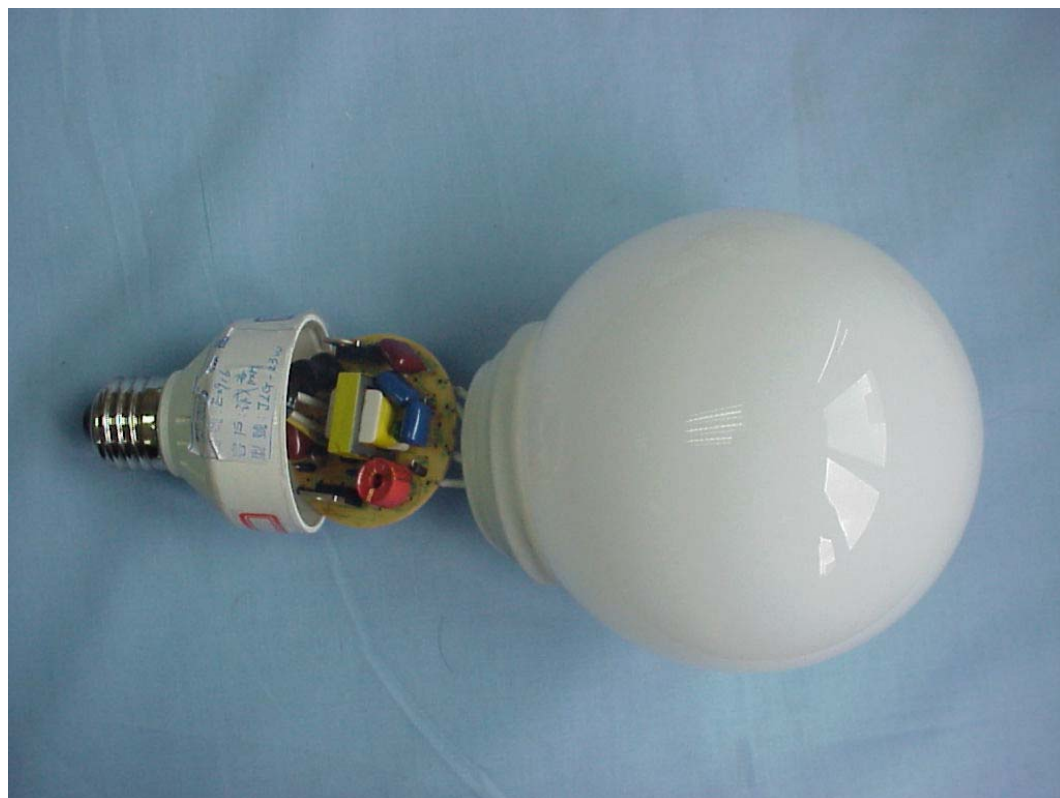
FIGURE 7 ENERGY SAVING LAMP (M/N: JLG-23W) COVER REMOVED
