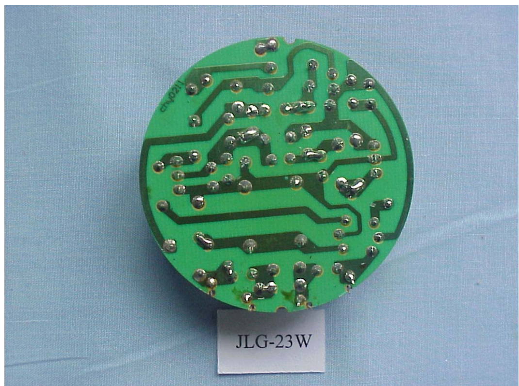
FIGURE 9 ENERGY SAVING LAMP (M/N: JLG-23W) MAIN BOARD (SOLDERED SIDE)
