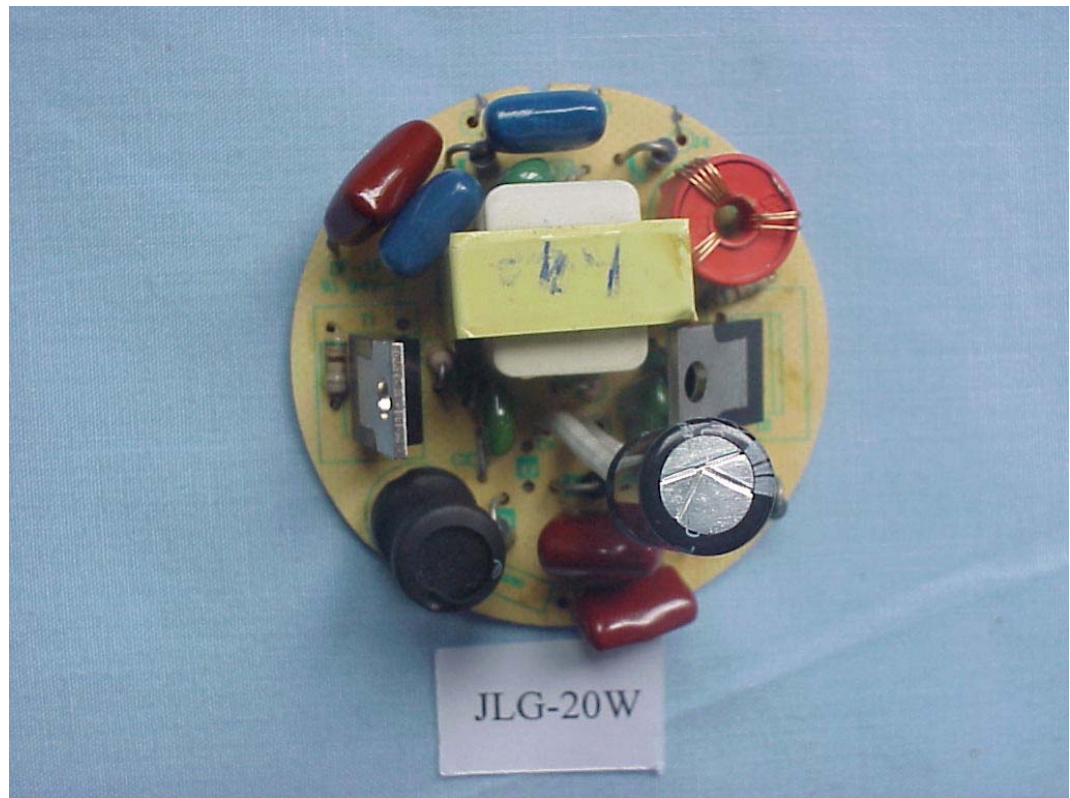
FIGURE 5 ENERGY SAVING LAMP (M/N: JLG-20W) MAIN BOARD (COMPONENT SIDE)
