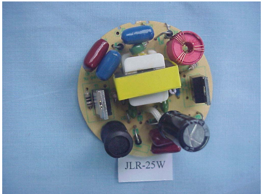
FIGURE 35 ENERGY SAVING LAMP (M/N: JLR-25W) MAIN BOARD (COMPONENT SIDE)
