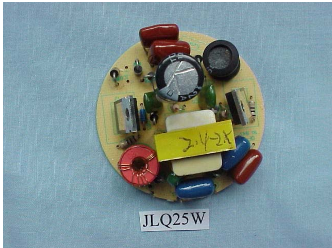
FIGURE 23 ENERGY SAVING LAMP (M/N: JLQ-25W) MAIN BOARD (COMPONENT SIDE)
