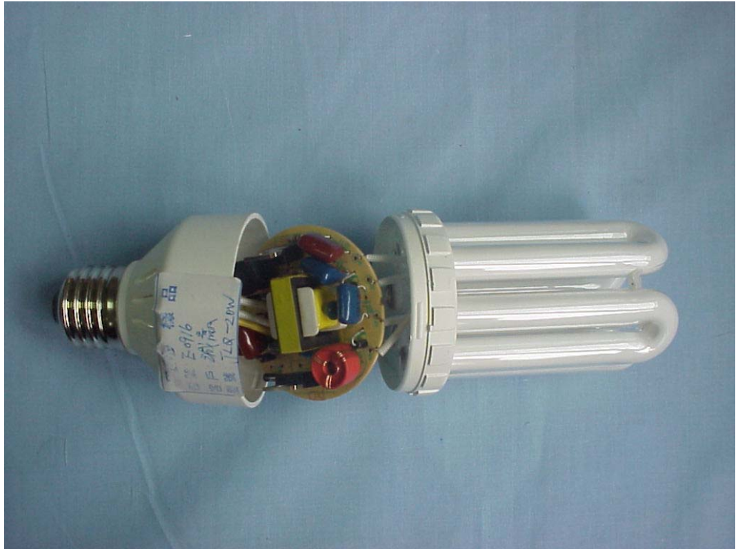
FIGURE 16 ENERGY SAVING LAMP (M/N: JLQ-20W) COVER REMOVED
