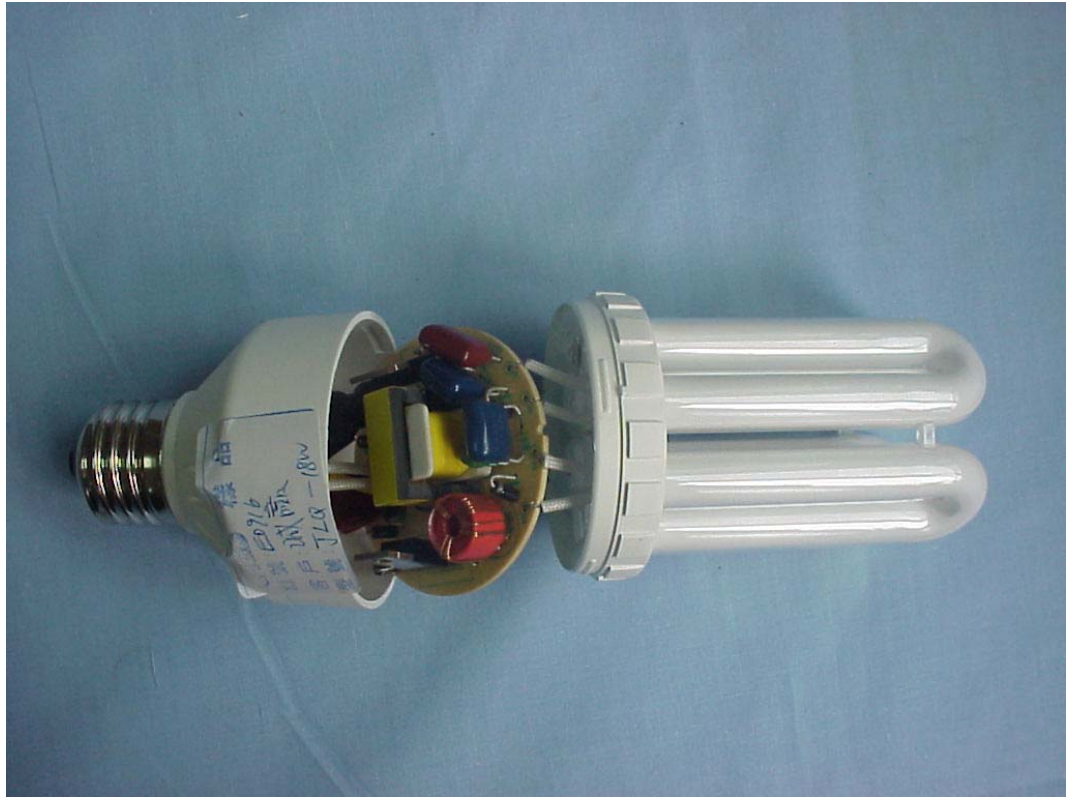
FIGURE 13 ENERGY SAVING LAMP (M/N: JLQ-18W) COVER REMOVED
