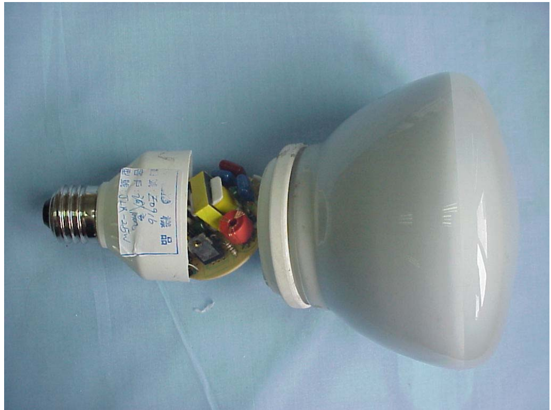
FIGURE 34 ENERGY SAVING LAMP (M/N: JLR-25W) COVER REMOVED
