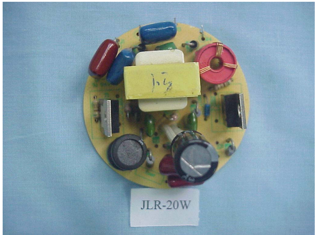
FIGURE 29 ENERGY SAVING LAMP (M/N: JLR-20W) MAIN BOARD (COMPONENT SIDE)
