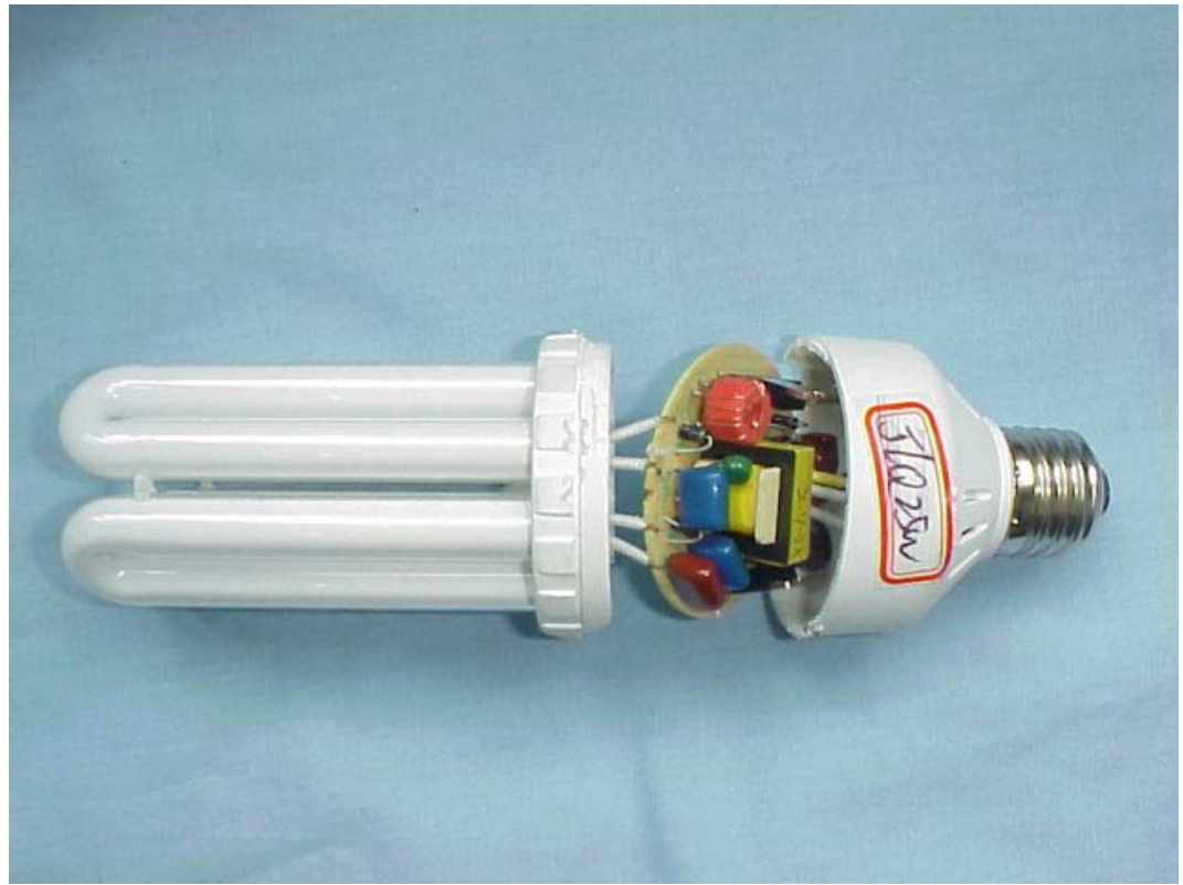
FIGURE 22 ENERGY SAVING LAMP (M/N: JLQ-25W) COVER REMOVED
