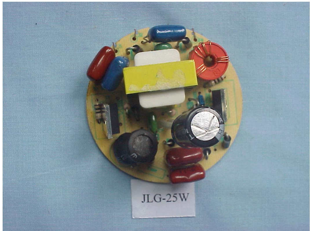
FIGURE 11 ENERGY SAVING LAMP (M/N: JLG-25W) MAIN BOARD (COMPONENT SIDE)
