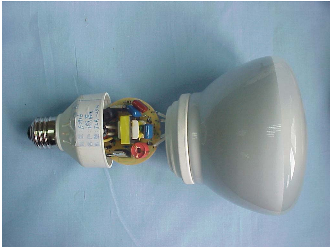
FIGURE 31 ENERGY SAVING LAMP (M/N: JLR-23W) COVER REMOVED
