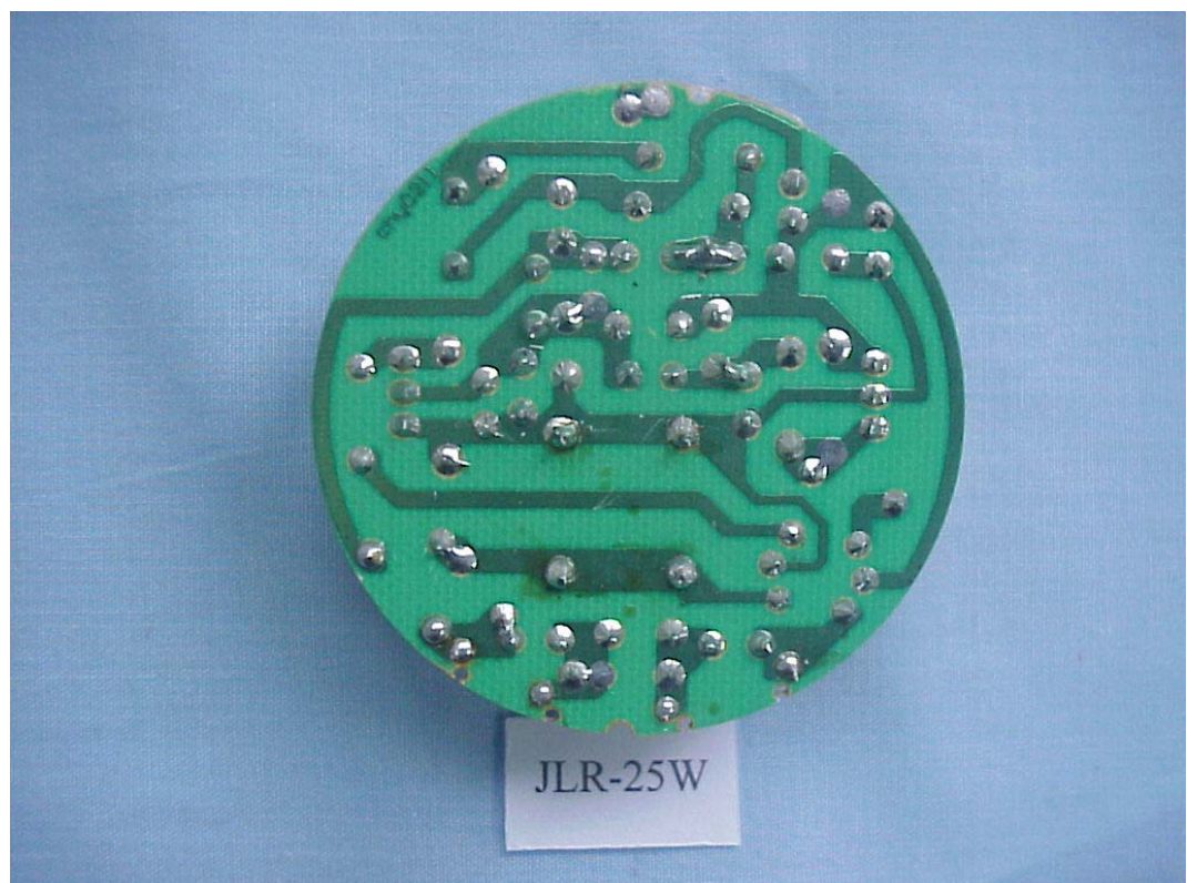
FIGURE 36 ENERGY SAVING LAMP (M/N: JLR-25W) MAIN BOARD (SOLDERED SIDE)
