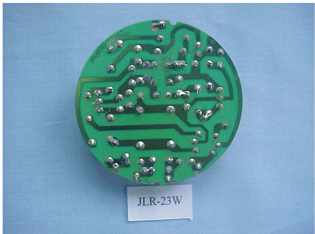
FIGURE 33 ENERGY SAVING LAMP (M/N: JLR-23W) MAIN BOARD (SOLDERED SIDE)
