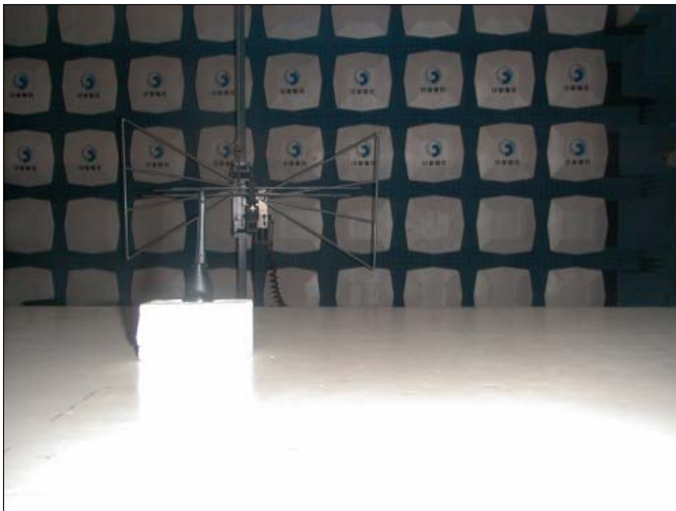
Test Setup for power measurement at 30~1000Mhz
