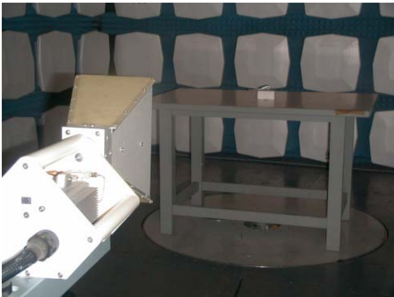
Test Setup for harmonic power
