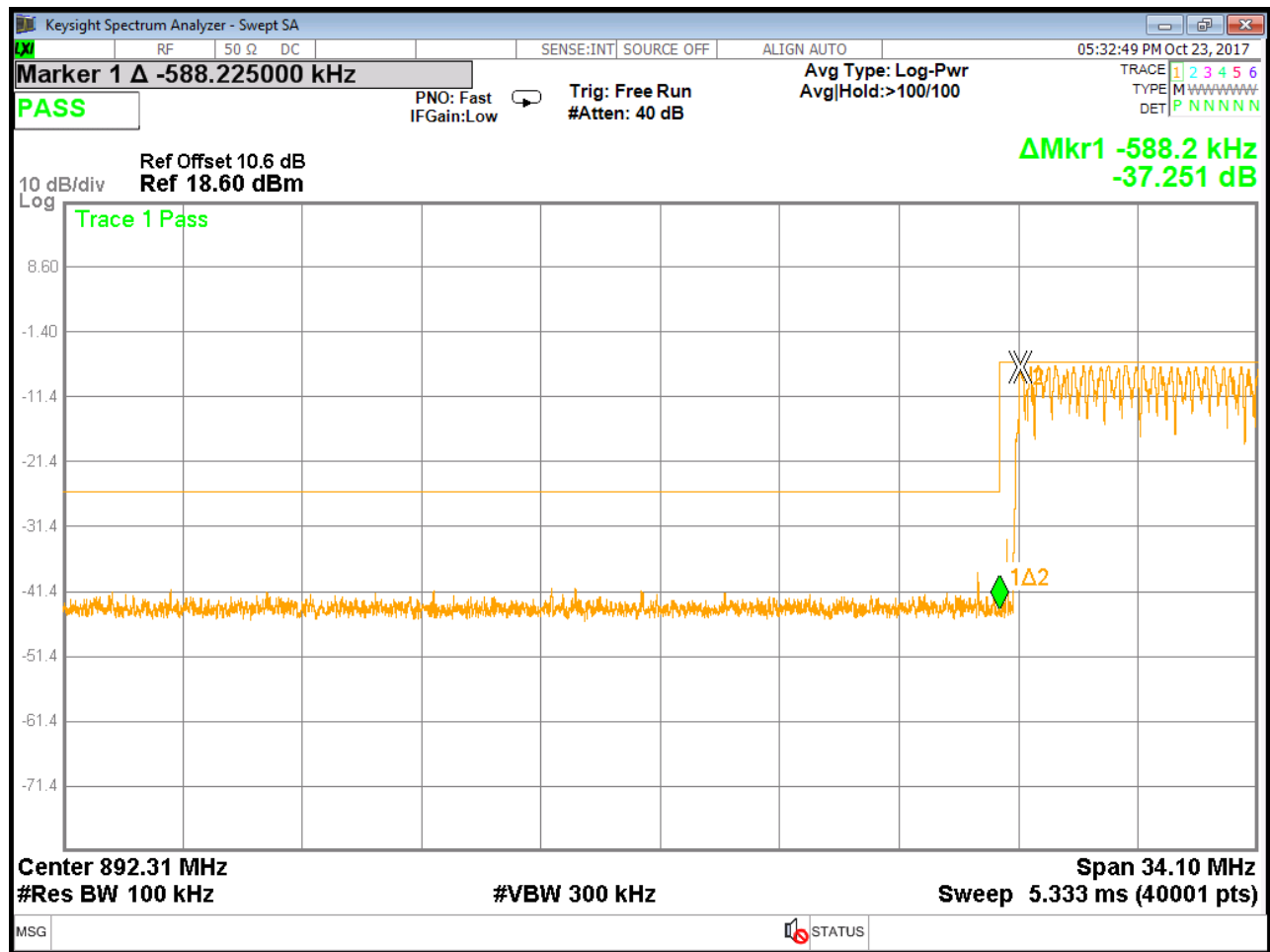
Figure 43: Low Channel, Lower Band-edge, Low Power Setting
