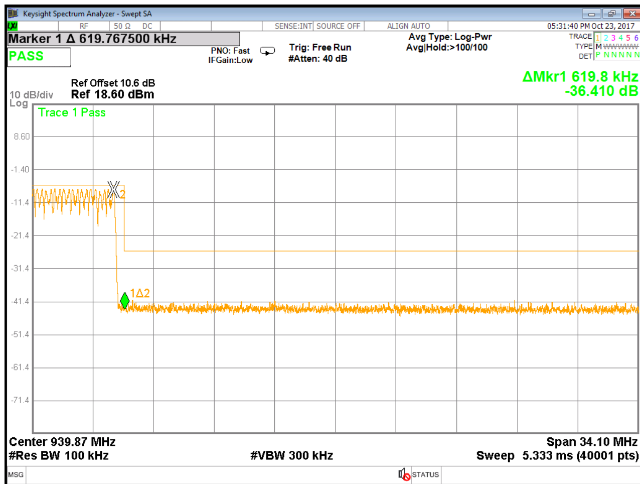
Figure 44: High Channel, Upper Band-edge, Low Power Setting
