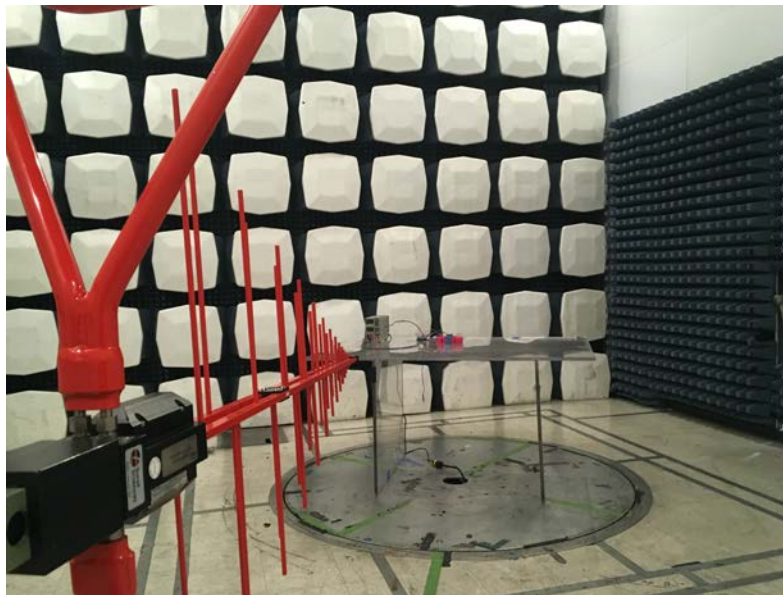
Photograph 3. Radiated Spurious Emissions, Test Setup, Below 1 GHz
