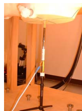
2450MHz System performance check setup
