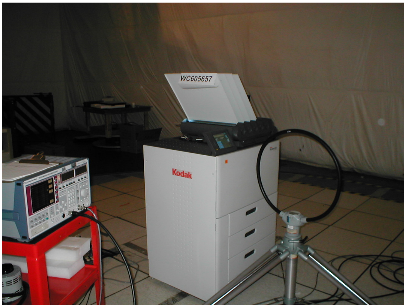
Test-setup photo(s): General Field Strength Limits 0.009 – 30 MHz
