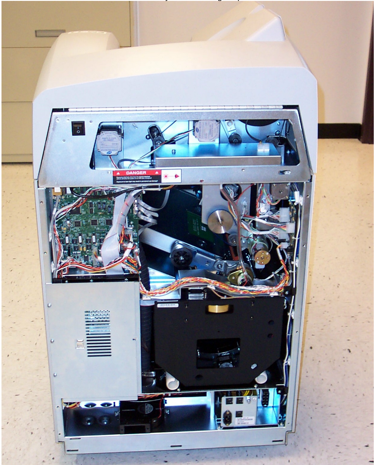
Disassembly - Rear of Imager Open
