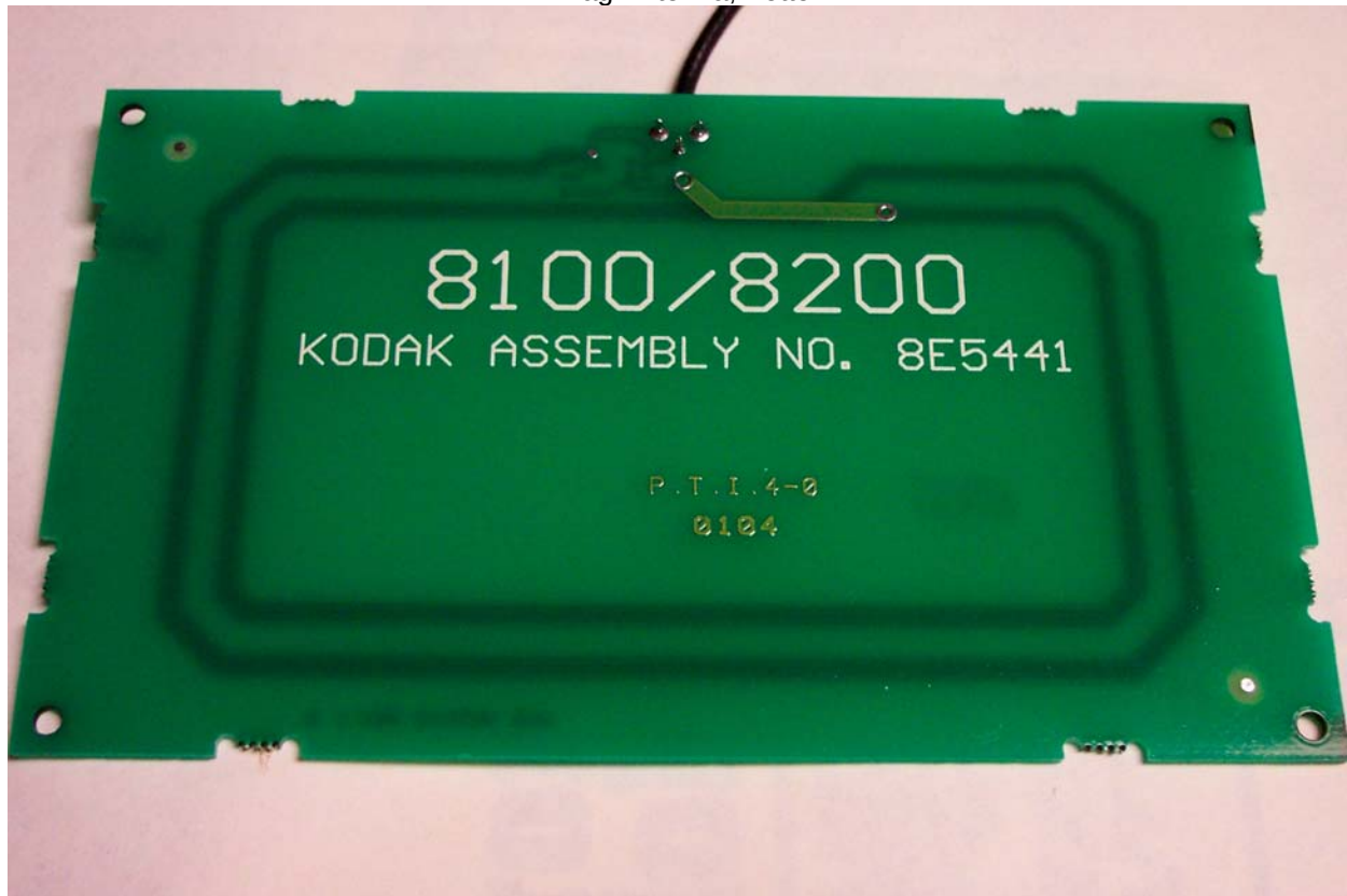
RF Tag Antenna, Bottom
