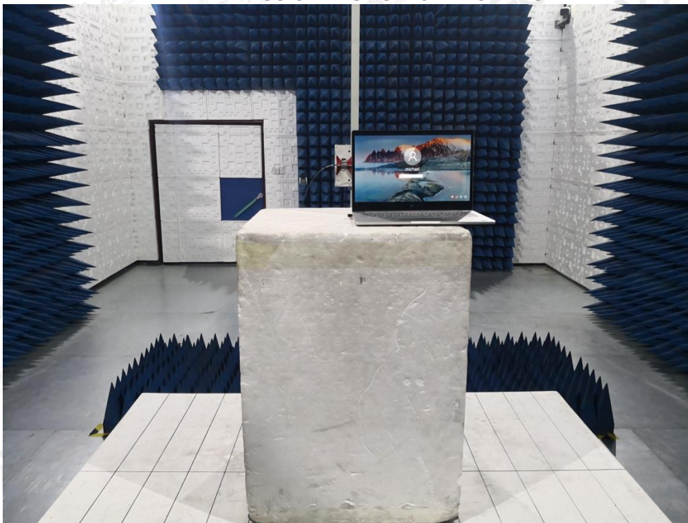
RADIATED EMISSION TEST SETUP ABOVE 1GHZ
