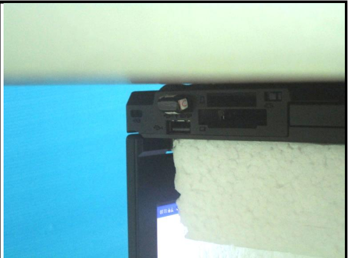
USB Horizontal Down with 0.5 cm Gap
