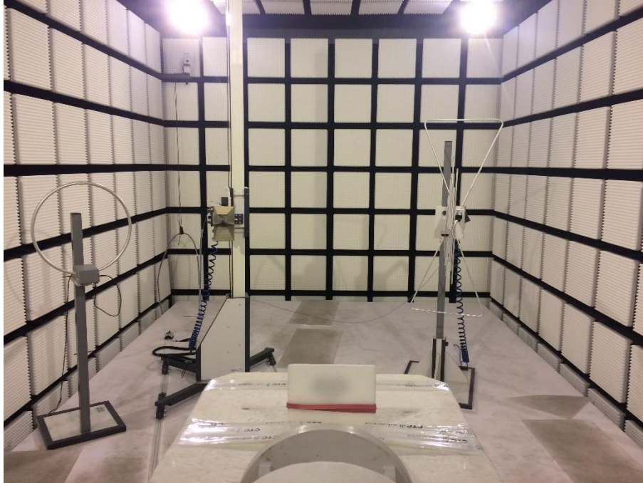
Photo 3: RSE set-up 1 GHz to 6 GHz
