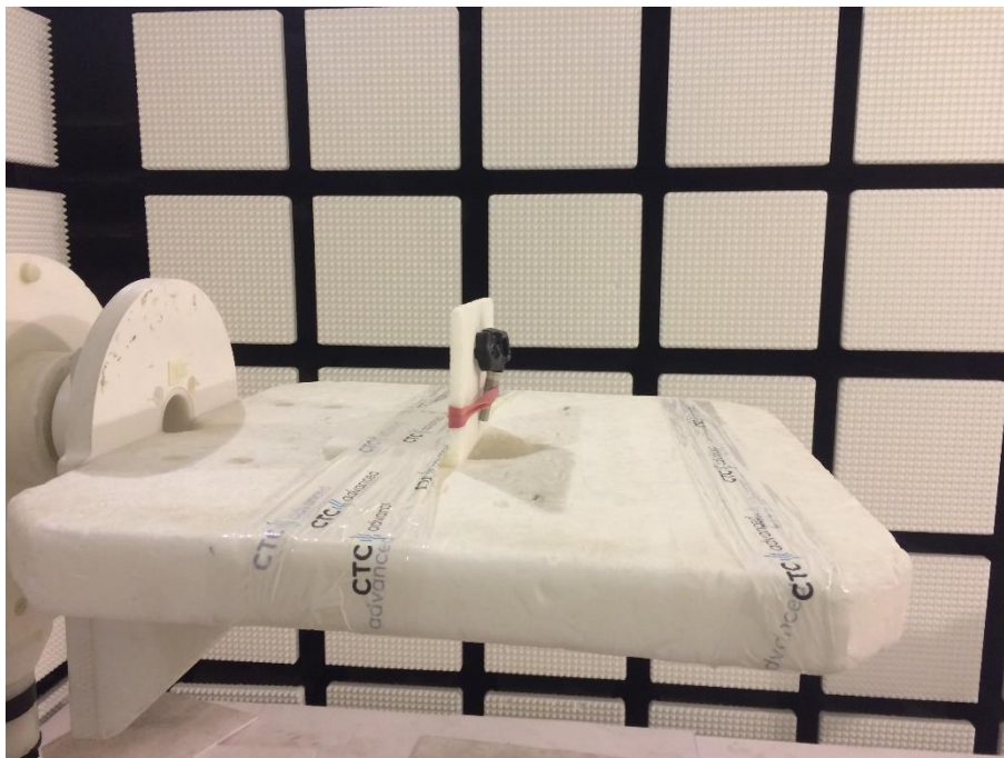
Photo 4: RSE set-up 1 GHz to 6 GHz
