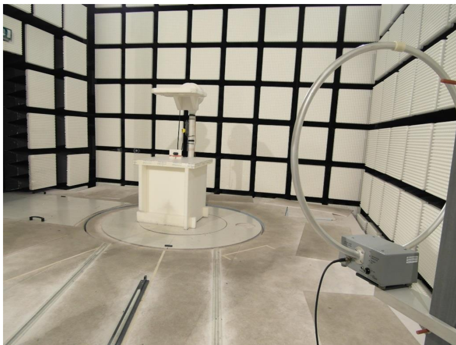
Photo 8: RSE set-up 9 kHz to 30 MHz
