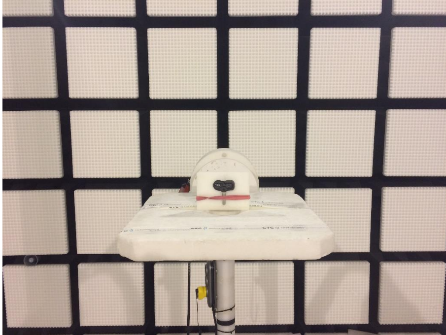
Photo 5: RSE set-up 1 GHz to 6 GHz
