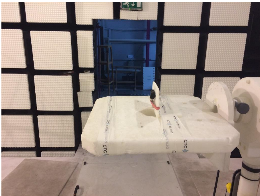
Photo 6: RSE set-up 1 GHz to 6 GHz
