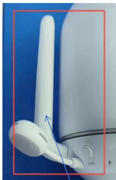
Copper pipe antenna
