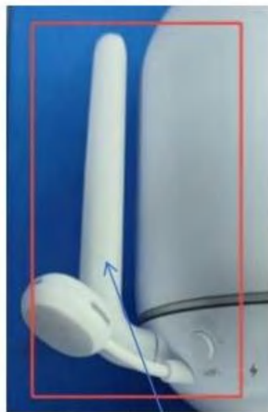
Copper pipe antenna
