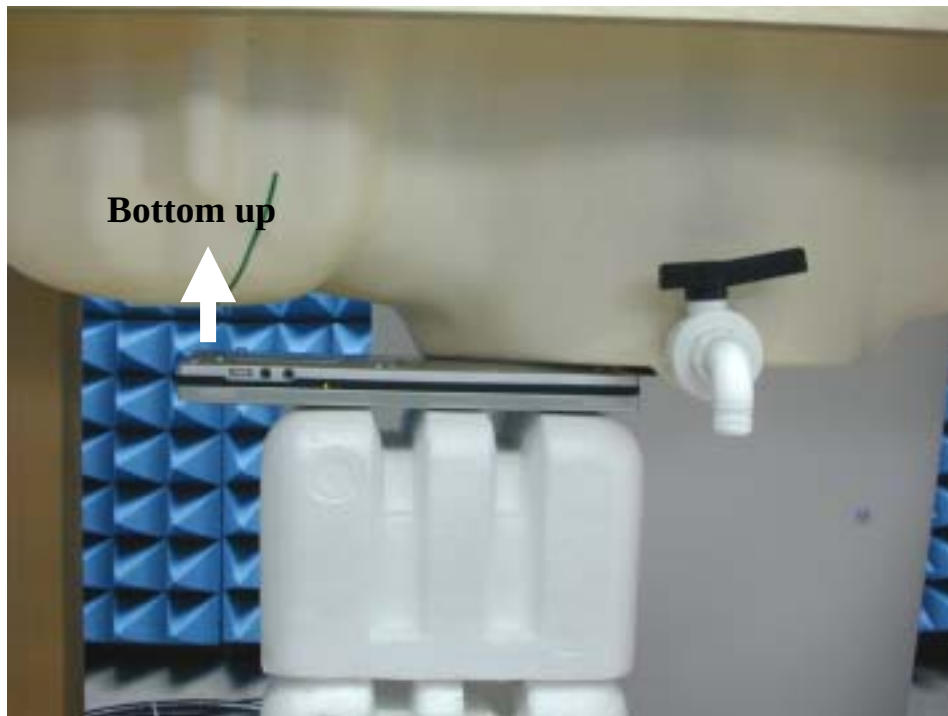
Fig.5 Photograph of the Bottom of the Pc is paralleled and at a distance of 0.0 cm from the base of the phantom.
