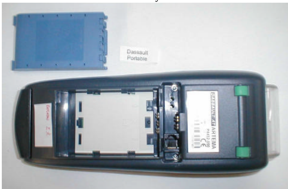
Bottom - Battery Removed
