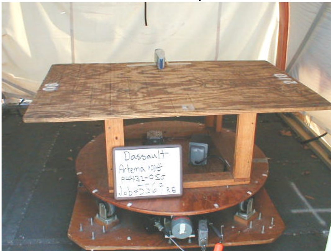
Radiated Emissions Test Setup – Back View
