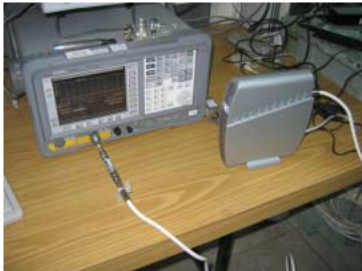
Photograph 7.1.3 Peak output power test setup
