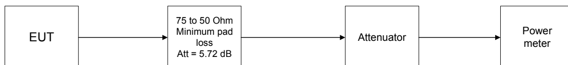
Figure 7.1.1 Peak output power test setup
