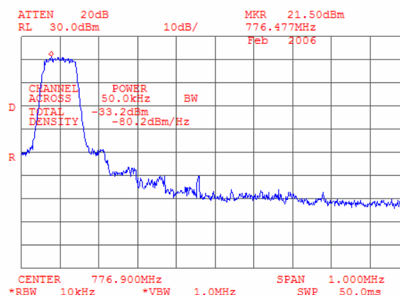
Plot 7.4.20 Adjacent channel coupled power measurements, mid carrier frequency, QPSK
